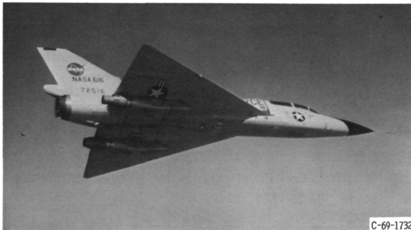
Figure 1. - Modified F-106B aircraft in flight, showing underwing installation of nozzles.
