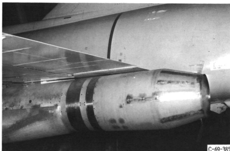
Figure 2. - Basic variable-flap ejector nozzle located under trailing edge of wing.
