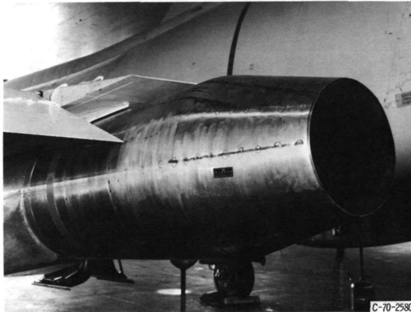
Figure 5. - Low-area-ratio variable-flap ejector nozzle located under trailing edge of wing with elevons deflected down.
